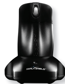
H Silver Storm Wireless Waterproof Mouse 2.40 GHz operating frequency. 1000 dpi movement resolution. Scroll wheel. 2 buttons. Charging stand. For right- or left-handed users. SSH STM042WE (841130)
